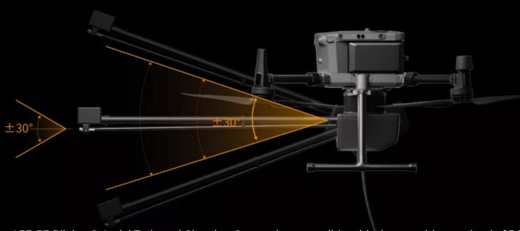
The Orion AP3-P3 Pliabot® Aerial Tethered Cleaning System is compatible with drones with a payload of 3-10kg (6-22lb). It offers an efficient and versatile high-pressure aerial cleaning solution for various scenarios, including building exteriors, solar panels, insulator strings, and tall structures.
