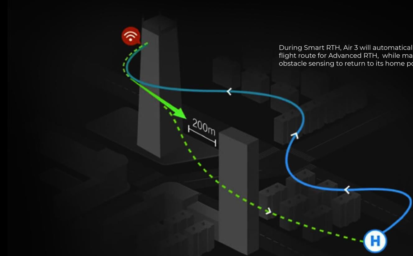
During Smart RTH, Air 3 will automatically plan an optimized flight route for Advanced RTH, while maintaining omnidirectional obstacle sensing to return to its home point quickly and safely.
