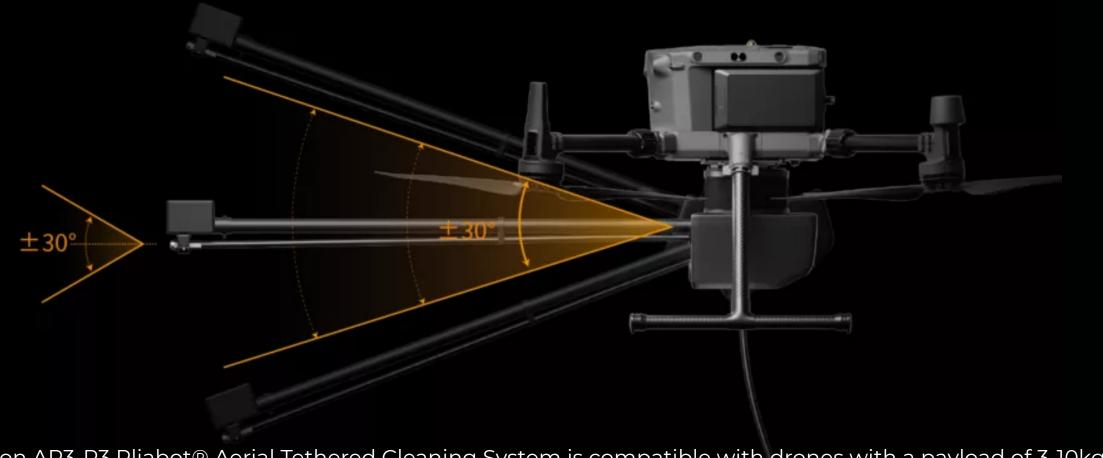
The Orion AP3-P3 Pliabot® Aerial Tethered Cleaning System is compatible with drones with a payload of 3-10kg (6-22lb). It offers an efficient and versatile high-pressure aerial cleaning solution for various scenarios, including building exteriors, solar panels, insulator strings, and tall structures.
